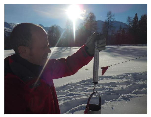
"Since decades the SLF is using Pesola spring scales to measure the snow water equivalent. We appreciate the precision, robustness and longevity of the scales. With the newly developed SWE-scale we were able to further improve the handling. Pesola proved to be an innovative and flexible partner", says Lukas Dürr, Technical Staff Member at the SLF.
